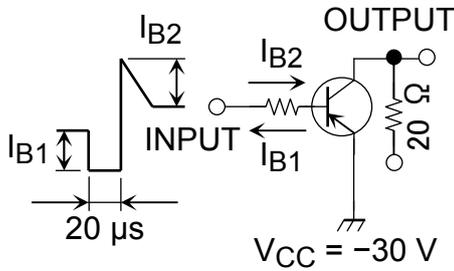
$I_{B1} = 75 \text{ mA}, I_{B2} = 75 \text{ mA},$
