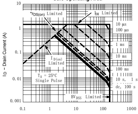
$V_{DS} > \text{minimum } V_{GS}$  at which  $r_{DS(on)}$  is specified
